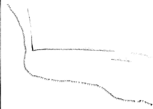
Figure 20: Reconstruction from the sequence 'Farmhouse', which contains long portions where a single plane fills the field of view. The successful reconstruction is a strong practical proof of the fact that the calibrated framework can overcome planar structure degeneracy without relying on the degeneracy or trying to detect it.
